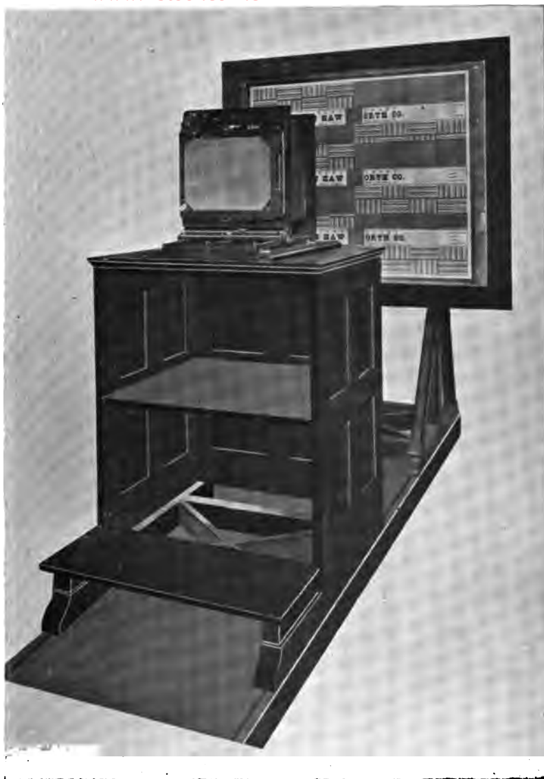
LENS-TESTING CHART SHOWING CAMERA, STAND, CHART AND PORTION OF PLATFORM.
