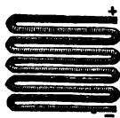
Figs. 16 and 17.—Nobili's Thermo-electric Battery.
