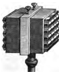
Figs. 16 and 17.—Nobili's Thermo-electric Battery.
