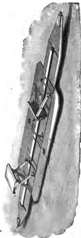
Sectional Bottom-board of 12-foot Boat. Showing Camp-stools and Side-boards.
