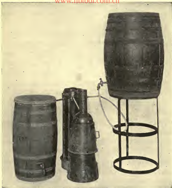
FIG. 21.—Forbes' sterilizer with "wood-burning attachment" and "barrel accessory."
