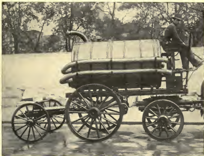
FIG. 31.—“Odorless excavator” tank wagon, with pump as a trailer.
