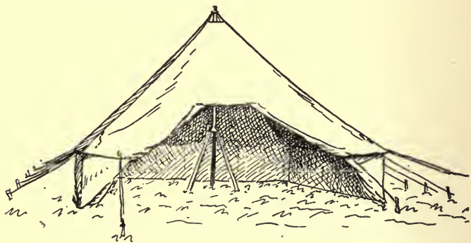
FIG. 49.—Pyramidal tent, with tripod support (United States Army standard model for fixed camps).
