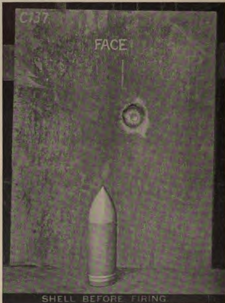
Hadfield "Era" Plate ( 3\frac{5}{16} in.), tested with 4\frac{1}{2} in. common shell (31 lb.), s.v. 2140 f.s., s.e. 988 ft.-tons.
