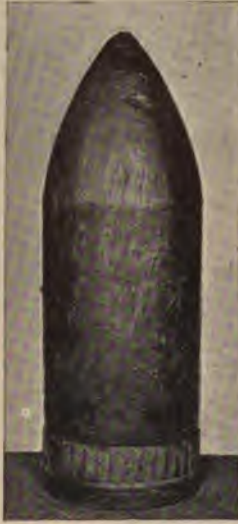
Hadfield 9.2-in. "Heclon" A.P. shell after perforating 11 in K.C. Plate, s.v. 2000 f.s.
