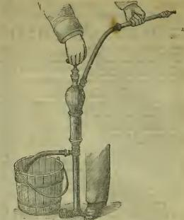
BARR'S PORTABLE GARDEN ENGINES. No. 1, 50/; No. 2, 42/.- No. I will throw a continuous stream of water 40 feet, and through a 3-inch suction-hose draw its supply from a distance of 60 feet. No. 2 will draw water from a distance of 30 feet through a 4-inch hose. These engines are constructed on the best principles. They are not liable to get out of order, while their value for washing wall fruit trees, cleansing hops, and watering flower-beds, etc., cannot be overestimated.
