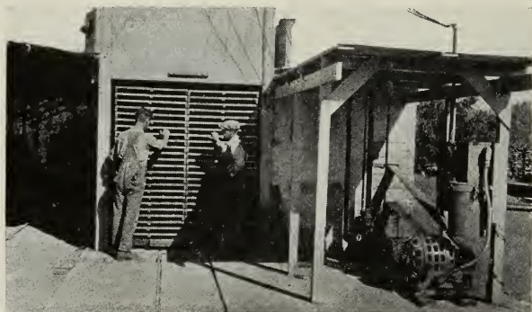
Fig. 2.—Placing a car of prunes in a tunnel dehydrater. Note how closely the stacks of trays fit the tunnel.
