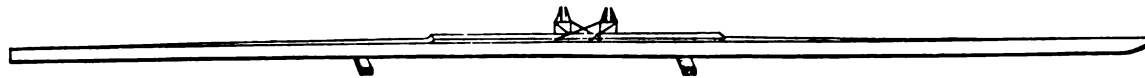
A SCULLING OUTRIGGER, 30 Feet Long. New Style for Racing in Smooth Water.
