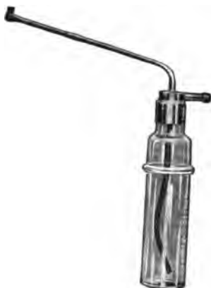
Fig. 170.—De Vilbiss spray tube, provided with an adjustable tip so that the spray may be thrown in any direction.
