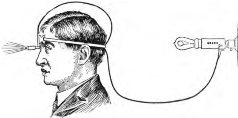
Fig. 8.—Electric magnifying headlight. This is a very simple, inexpensive, and very satisfactory electric headlight. It may be used either on the street current or vest-pocket battery. It is very light, compact, and can be so adjusted that the light is brought between the operator's eyes. There is a condensing lens which assists in focusing, thus greatly increasing its efficiency.
