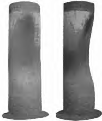
COLLAPSED FLUE OF DONKEY BOILER.
