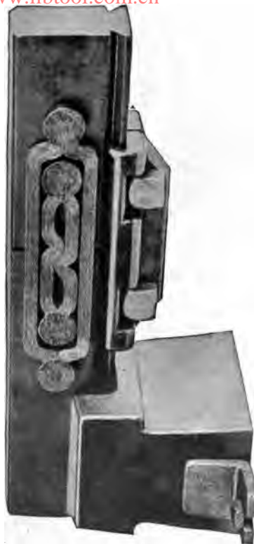
Fig. 357. Third Rail, Insulator, Connector and Riveted Bond.
