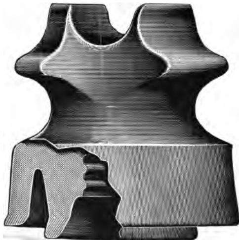
Fig. 337. Glass Cable Insulator, 10,000 Volts.
