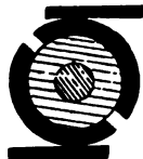
Fig. 188. Cross Section of Simple Commutator. Black Represents Copper; White Space Is Mica Insulation.
