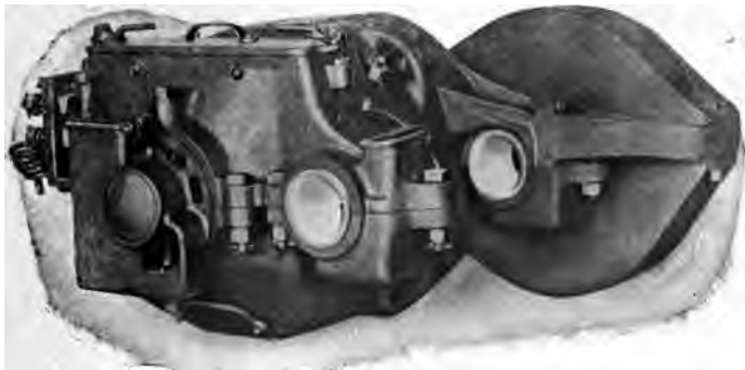
Fig. 221. D. C. Railway Motor, 40 H. P.
