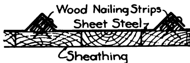
Fig. 17. Method of Laying Sheet Steel with Crimped Edges.
