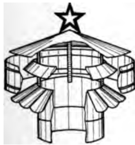
Fig. 69. Details of "Star" Ventilators.
