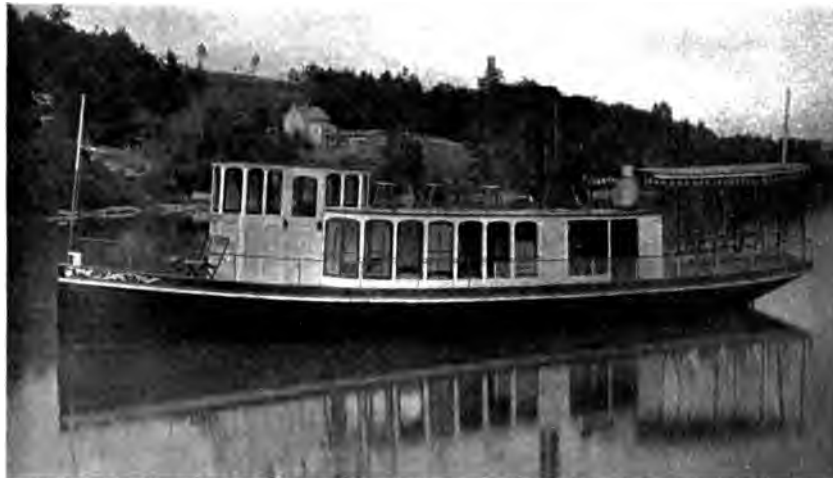
T. H. Worrall's steam yacht Gracie . Fifty feet long, ten feet wide.
