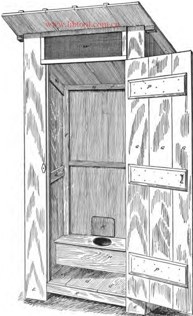
Fig. 38.—Front view of single-seated sanitary privy. (Redrawn from Stiles.)
