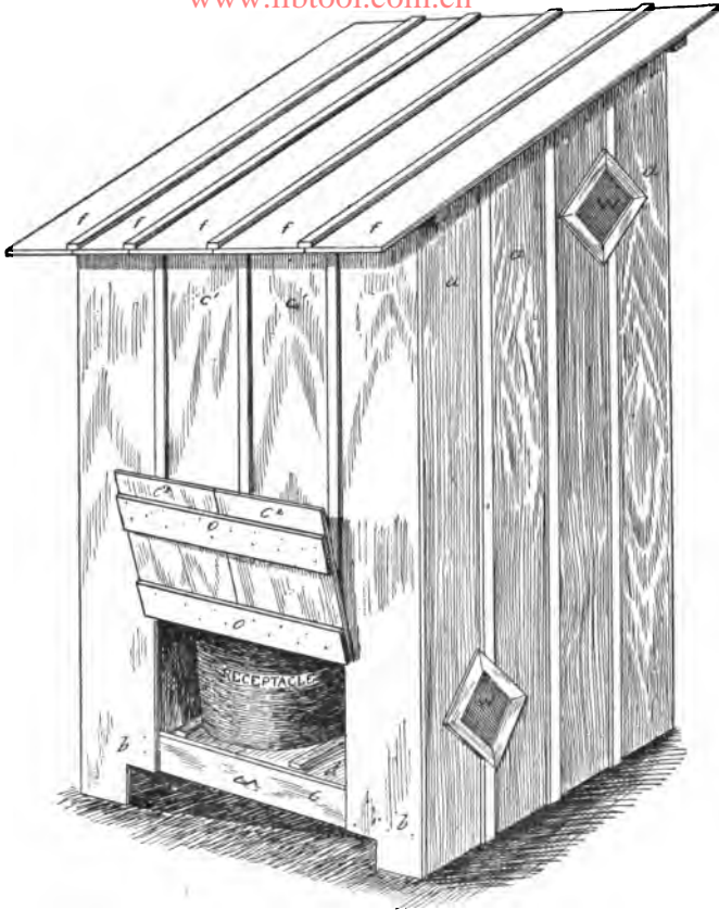
Fig. 39.—Rear view of single-seated sanitary privy. (Redrawn from Stiles.)
