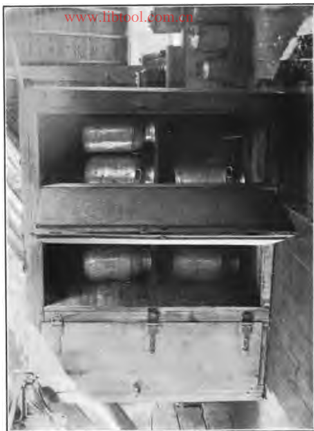
STEAM BOX FOR STERILIZING CANS.
