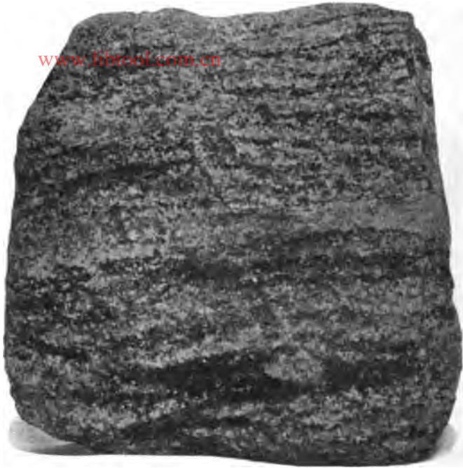
FIGURE 3.—Gneiss from Leete Island Quarry. Showing gneissoid texture due to squeezing and stretching of granite.
