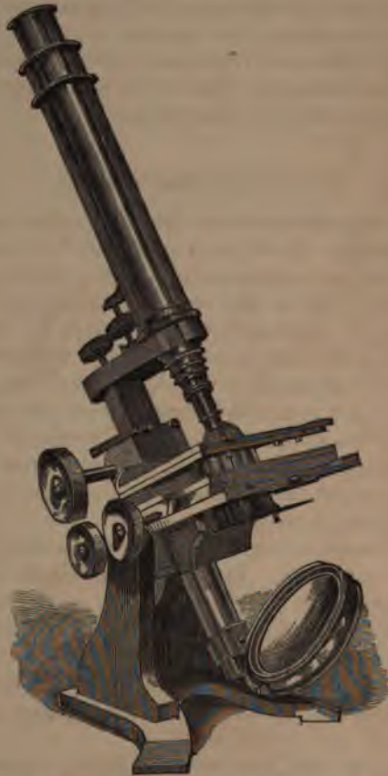
fig. 35. Baker's Compound Microscope.
