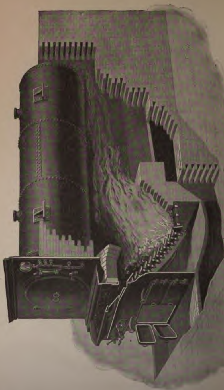
GENERAL PERSPECTIVE OF THE RONEY MECHANICAL STOKER AS APPLIED TO A HORIZONTAL TUBULAR BOILER.
