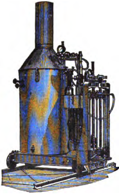
FIG. 15.—DIAMOND CHANNELLING MACHINE.
