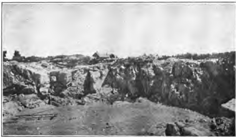
A. QUARRY OF THE OZARK STONE COMPANY AT OZARK, MACKINAC COUNTY. The massive bedding and the irregular jointing are characteristic of the Engadine dolomite.
