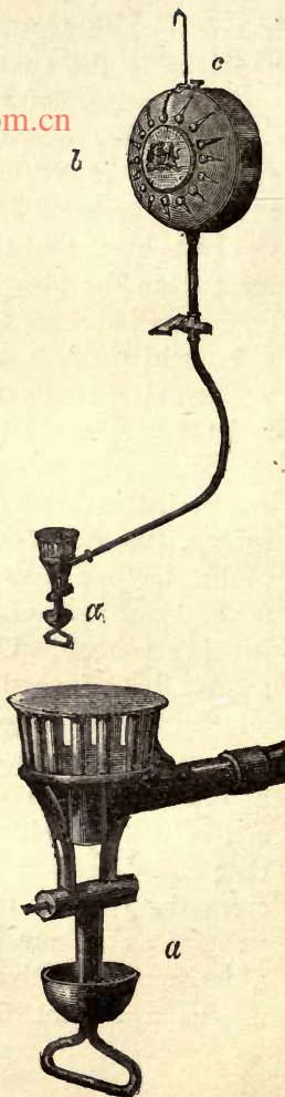
FIG. 4.—Read Holliday's lamp for burning light coal-tar oils. The oil is contained in the cistern c , from whence it flows down the pipe, when the stopcock is opened, into the burner a . Below the burner is a little cup, in which some of the oil is kept burning, and the heat from this flame volatilizes the oil as it flows down the pipe, the vapour thus generated issuing from the jets in the burner and there undergoing ignition. The burner and cup are shown on an enlarged scale at a in the lower figure.
