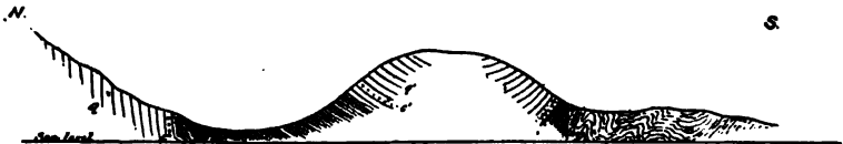
FIG. 6.—Section across valley near Ashleam Bay, showing quartzite ( q ) with pebbly grits on either side, micaceous and graphitic schists, and coarse dark-gray grit beds between: also mica-schist ( m ) faulted up against corresponding rocks south of the central hill.
