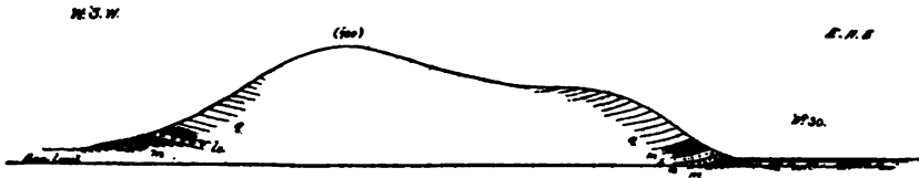
FIG. 5.—Section across Glencastle Hill and Carrowmore Lough (Wr. 30), showing mica-schist ( m ), limestone ( ls ), and pebbly deposit ( b ), under quartzite ( g ).
