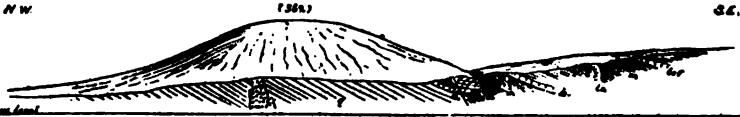
FIG. 4.—Detailed section at Glencalry, showing quartzite ( g ) invaded by epidiorite, over-ridden by mica-schist ( m ) and limestone ( ls. ), along reversed fault.
