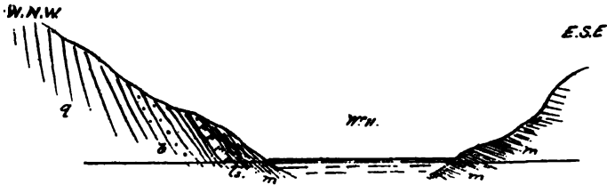
FIG. 9.—Section across Lough Feeagh (W.11) showing quartzite ( g ), pebbly beds ( b ), limestone ( l ), and mica-schist ( m )—natural order of succession inverted.
