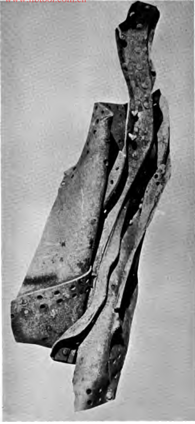
DAMAGED SHIP PLATE FROM S.S. "ROTTERDAM."
