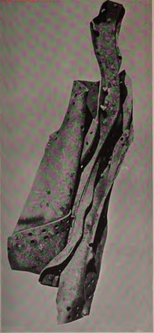
DAMAGED SHIP PLATE FROM S.S. "ROTTERDAM."
