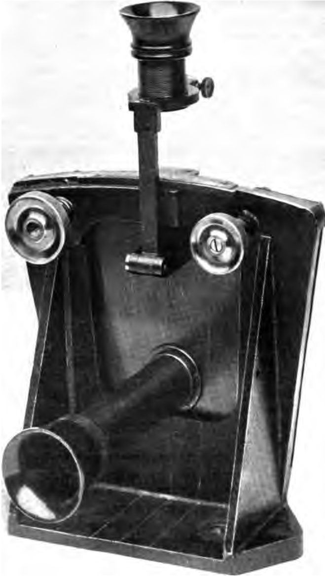
FIG. 11.—TORQUE FINDER OF FLASHLIGHT TORSION-METER (BEVIS
