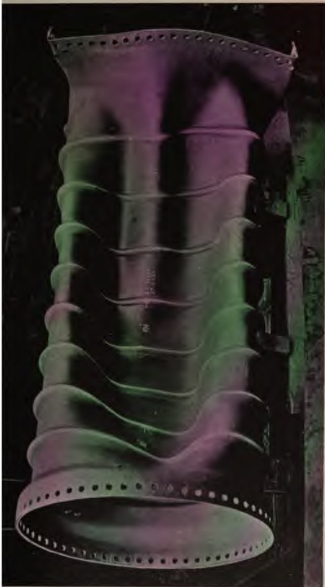
OVERHEATED BOILER FURNACE.
