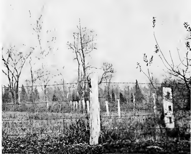
4. Lens Test No. 2. Same subject, distance, plate, and date as Test No. 1. Front lens (fourteen-inch focus) of Zeiss Convertible, No. 10; diaphragm F. 16; \frac{1}{25} second.
