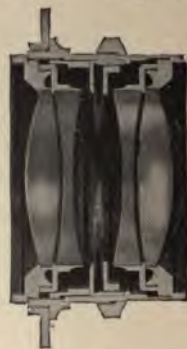
FIG. 38. Double Anastigmat. C. P. Goerz Optical Works.
