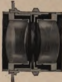
FIG. 14. Double Anastigmat Lens. C. P. Goerz Optical Works.
