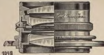
FIG. 41. "Tessar" Lens. Carl Zeiss.
