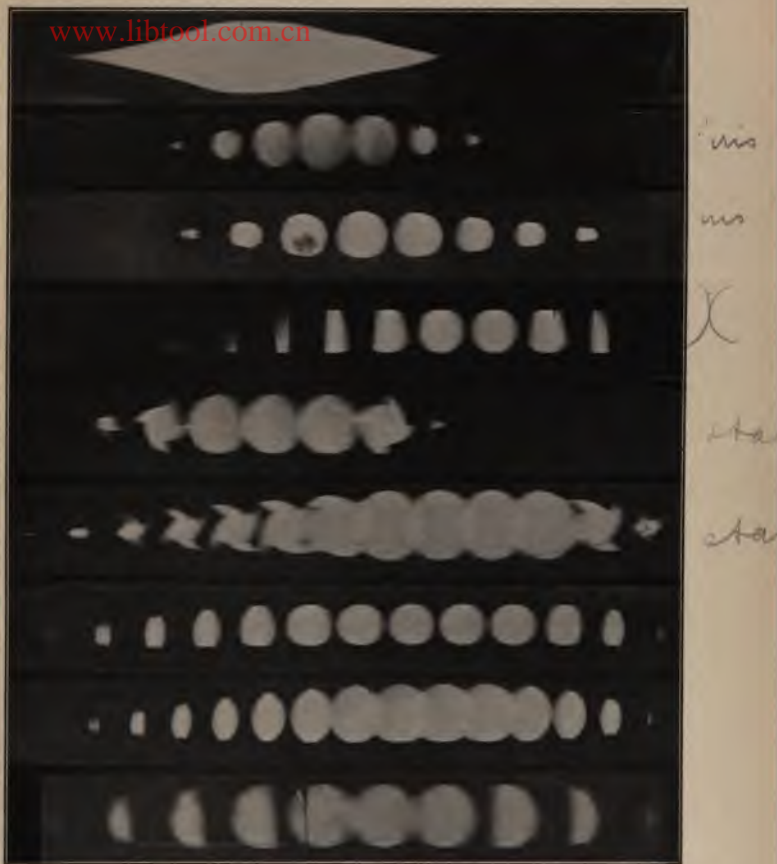
FIG. 85. Shutter Apertures during Exposure.
