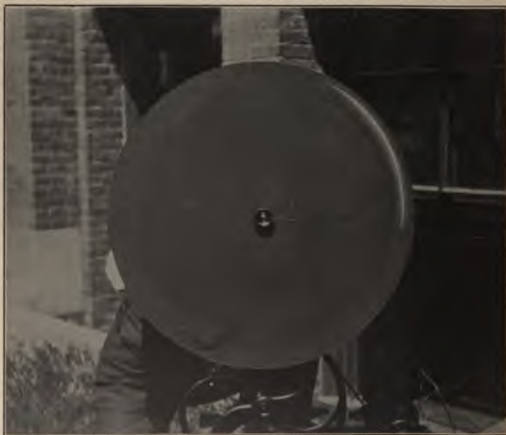
FIG. 83. Test of Shutter Exposure Time.
