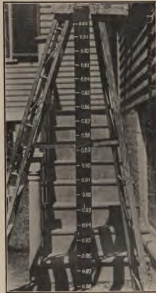
FIG. 84. Test of Shutter Exposure Time.
