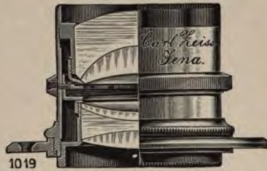
FIG. 36. "Protar" Lens. Carl Zeiss.
