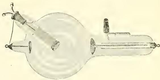
FIG. 4123. Water-Cooled Tube.
