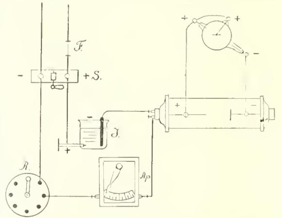
FIG. 4125.—Diagram of Installation of Apparatus with Electrolytic Interrupter. S, Switch; F, safety fuse; R, rheostat; A<sub>1</sub>, amperemeter; I, electrolytic interrupter.
