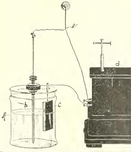
FIG. 4121.—Electrolytic (Wehnelt) Interrupter. *a*, Interrupter; *b*, platinum wire in porcelain cylinder; *c*, lead plate; *d*, coil; *e*, wires connecting interrupter and coil with an electrical source.
