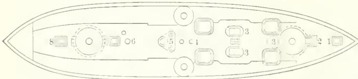
FIG. 3505.—Shows the Plan of the Upper Deck of the *Hoche* with its Eight Hatches, Marked by Treble Lines. Four small ones are in the centre line of the deck, and the four large ones (engine-room hatches) are arranged symmetrically by twos on each side of the centre line of the deck. (From Rochard et Bodet.)
