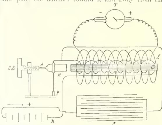
FIG. 4117. Diagram of Induction-Coil Apparatus with Vibrating Hammer Interrupter. A, Contact; B, battery; S, secondary; C, soft-iron core; H, hammer; c, condenser; T, tube.
