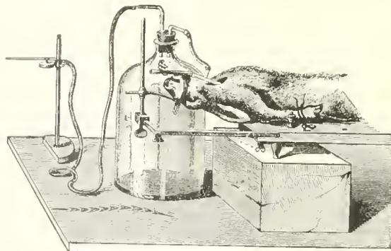
FIG. 4106.—Arrangement of Tracheal Cannula and Marec's Tambour for Recording Changes in Intrapulmonary Pressure. (Langendorff.)
