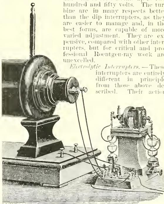
FIG. 4119. Coil with Mercury Dip Interrupter.
