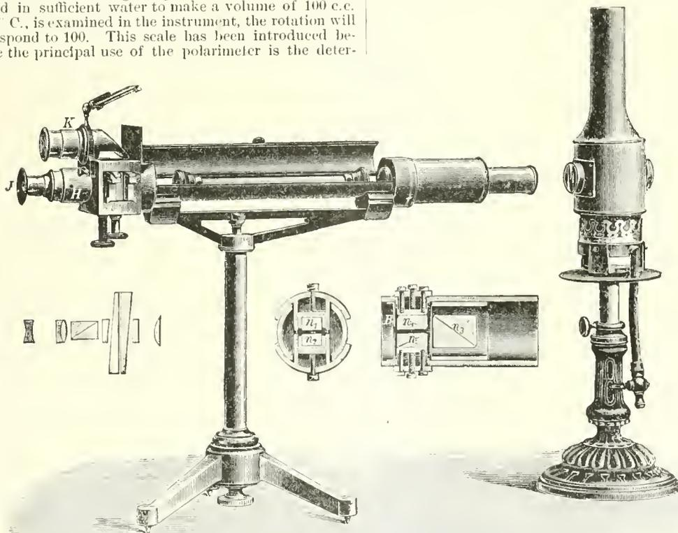
FIG. 3874.—Triple Field Polarimeter with Details of Polarizing and Analyzing Apparatus. (With permission of Eimer & Amend, New York.)
