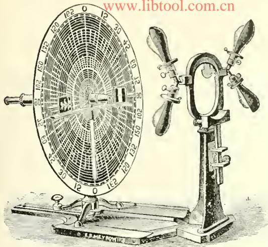
FIG. 3642.—Javal's Ophthalmometer with Attachment for Electrical Illumination of the Targets.
