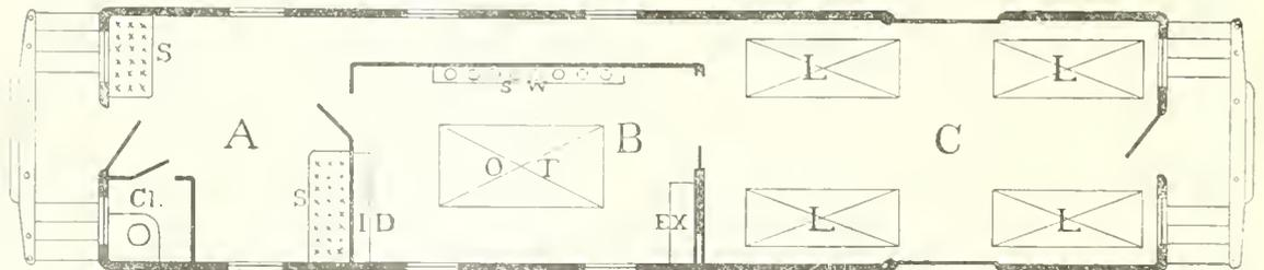
FIG. 3925.—Floor Plan of a Hospital Car. A, Sitting-room; B, operating-room; C, transportation-room; Cl., closet; S, seats; ID, instrument and dressing case; O.T., operating table; S.W., sterilized water and solutions, in racks; EX, extra sheets, blankets, and other materials; L, L, beds. (Herrick's "Railway Surgery.")
