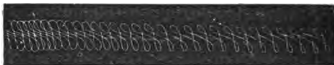
Trace of a Wheatstone's octave rod.
