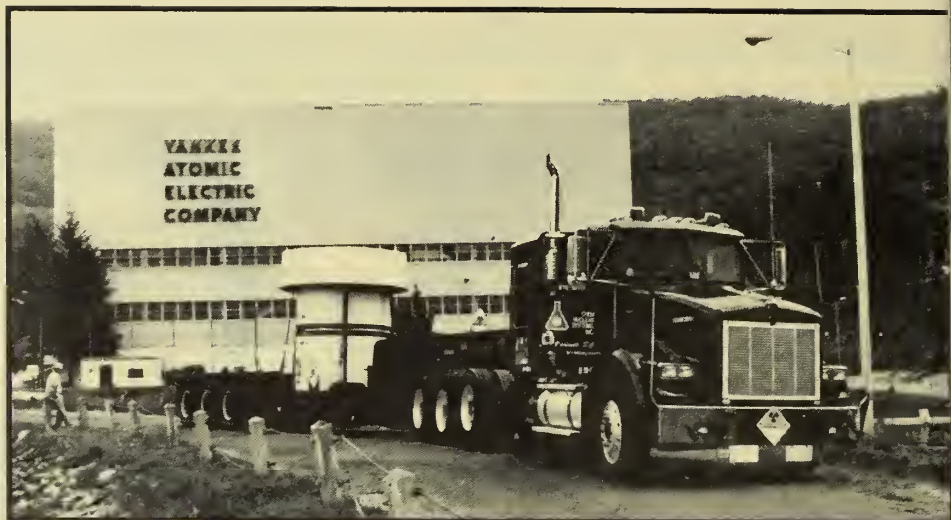
This shipment of LLRW, packaged in a cylindrical cask and tied down on a flatbed for truck transport, was typical of shipments from Yankee Atomic Electric Company's Rowe nuclear power plant to an LLRW disposal facility in Bamwell, South Carolina. A public forum on LLRW and high-level radioactive waste transportation will be held on April 7.
