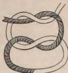
FIG. 80.—Method of tying square or reef-knot.
