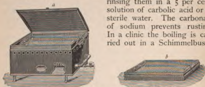
FIG. 18.—Schimmelbusch's gas-heated apparatus for sterilizing instruments: a, wire basket.
