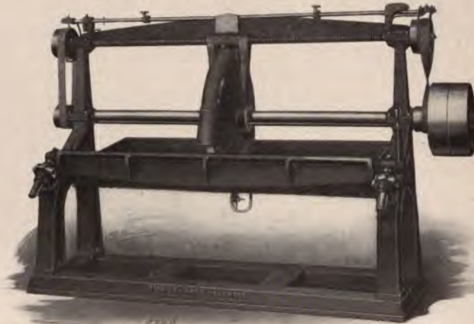
Rowe Straight-line Automatic Book Trimmer. (Capacity 24 packages of 4\frac{1}{2} or less in. thickness per minute.)
