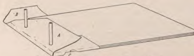
A — Leather back. B — Turn-in. C — Joint.
