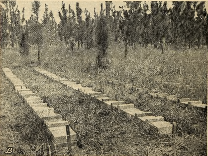
FIGURE 6.—Method of testing poisoned fiberboard in a trench between bricks and covered with bricks: A , Fiberboard samples set in between bricks; B , the rows of test samples covered by other bricks. Saucier, Miss., 1938.
