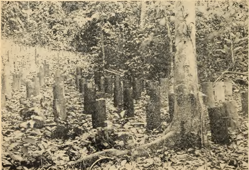
FIGURE 3.—Test of sections of impregnated pine telegraph poles in the ground on Barro Colorado Island, Canal Zone.
