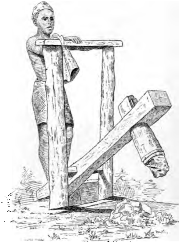
OPERATION OF FOOT-POWER MILL. QUARTZ CRUSHER AS USED IN THE MALAY PENINSULA.
