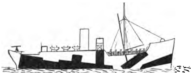
FIG. 15.—A camouflaged ship. It will be observed that a vessel so painted would, from a distance of several miles, give the appearance of a ship sinking while headed in the opposite direction.
