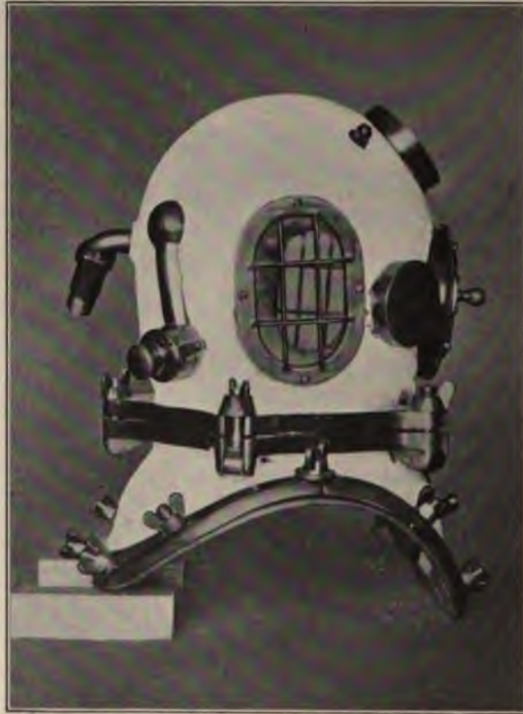
FIG. 25.—Standard Diver's Helmet, U. S. Navy. (Side view.)
