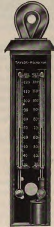
FIG. 2.—A type of Hygrometer (Mason) in common use.
