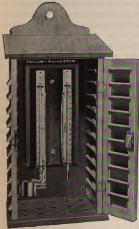
FIG. 1.—The Ship's Psychrometer.
