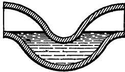
FIG. 39—Siphon water trap recommended by the General Board of Health, of England.
