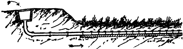
FIG. 275.—Plain hopper for slop-water disposal.
