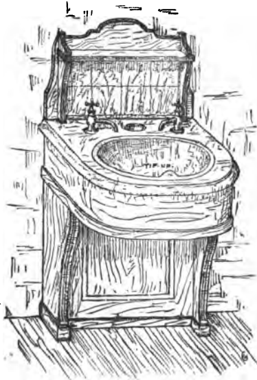
FIG. 247.—Open Cabinet-work for a Lavatory.
