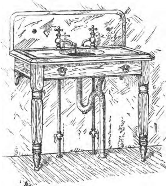
FIG. 246.—Open Arrangement for Wash-basins; slab supported on a frame resting on turned legs.
