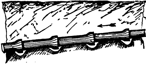
FIG. 265.—Proper method of laying earthen drains.
