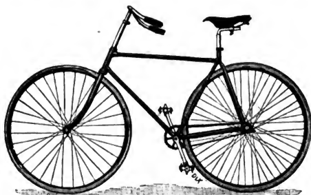
FIG. 1. "HADLEY" BICYCLE, FITTED WITH PNEUMATIC TYRES.
