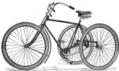
FIG. 2. "HADLEY" TRICYCLE, FITTED WITH PNEUMATIC TYRES.
