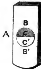
A—Outside frame of shutter. BB—Circumference of lenses. C—Half of the circumference covered up, marking half of the lenses. C'—The open part of lenses, equal to the other half which is covered.
